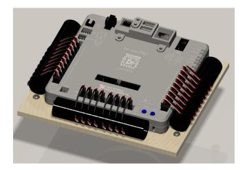
Team 868 was handpicked to beta test the RoboRIO, a new electronic controller being introduced in the 2015 kit of parts. The RoboRIO replaces both the bulky cRIO and Digital Sidecar, and doubles the number of PWM cables that can be used. Electrical Lead,
